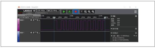
Figure 3-3 Logic analyser capture result (incomplete preamble)
